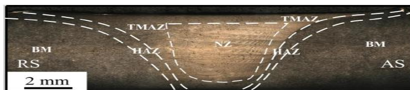
Fig.10 : The macro cross-section of the whole weld
