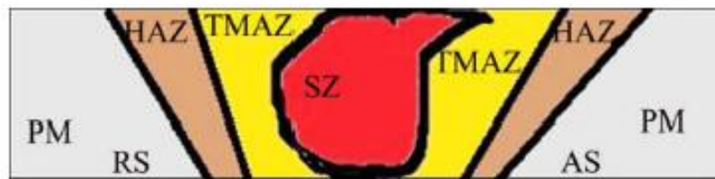
Fig. 7: Different Characteristic Zones of FSW/UFSW
